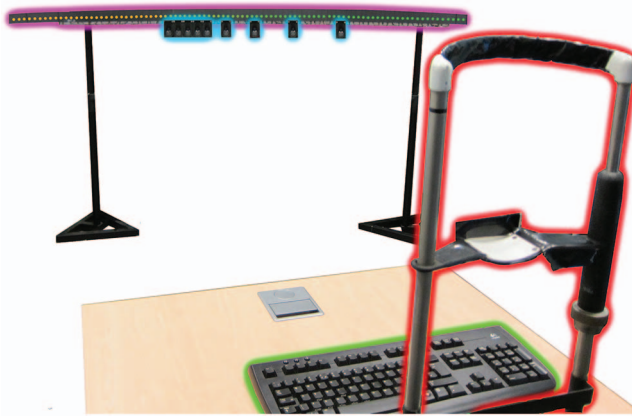
Figure 1. The ring of LEDs and speakers. On each presentation a flash of lights from a subset of LEDs and/or a noise from a speaker was presented. Participants maintained their head position fixed at straight ahead, using a chin rest, and entered responses using the keyboard. See the online article for the color version of this figure, in which LEDs, speakers, chin rest and keyboard are outlined in purple, blue, red, and green respectively.
